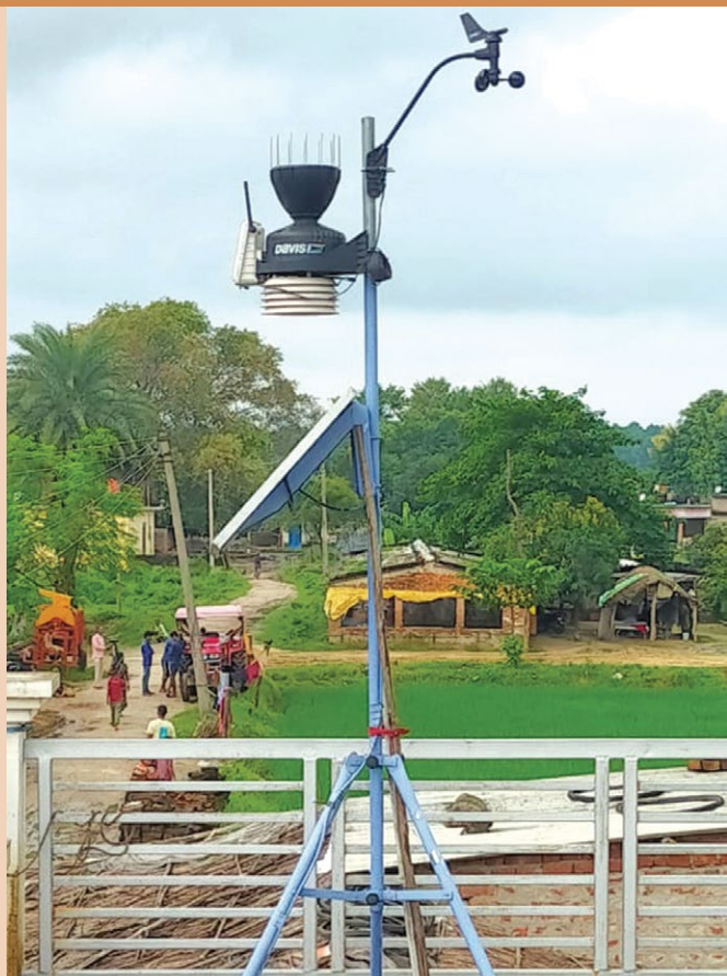
Automatic Weather Station collecting and processing weather data
